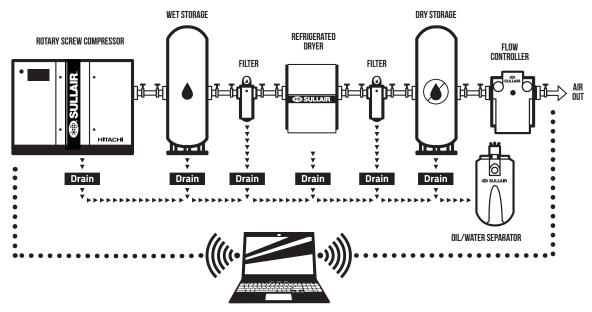
Hitachi Global Air Power offers total compressed air systems to help compressed air users reduce energy costs and improve productivity by analyzing, managing and controlling their compressed air systems.
