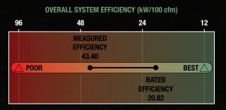
Specific Power (kW/100 cfm) is a normalized performance metric for representing the efficiency of a compressed air system. The graphic on the bottom right provides a snapshot assessment of the maximum potential performance of your system — the Rated Efficiency — compared to its actual Measured Efficiency.
