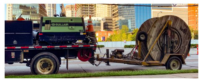
Compressed air is everywhere. Portable diesel air compressors bring compressed air wherever it is needed: plantside, roadside, refineryside and many other jobsites.
