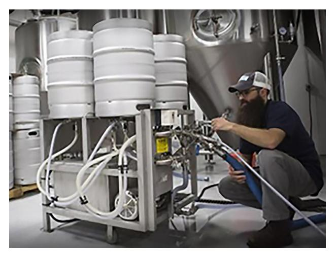
When speaking with a microbrewery, we learned about other usage of the compressed air. Many breweries use the compressed air for cleaning and canning applications. When washing kegs, breweries use compressed air to push cleaning agents through the keg washing process. In addition, it is used for keg purging after sterilization.
